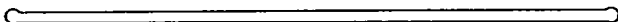
Fig. 2. Tube profile for minimization of end-effect. D_1 \rightarrow D + 0.0190 \cdot v_0^2 z_0^2 / D .
